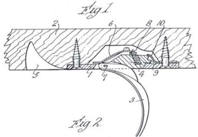
Athol Purdey's trigger designed to be used on a walking stick.
